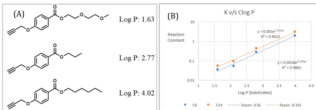
**Figure 3:** A. Structures of substrates with different  $\log P$  values. B.  $k$  vs  $\text{Log P}$  of substrates.
