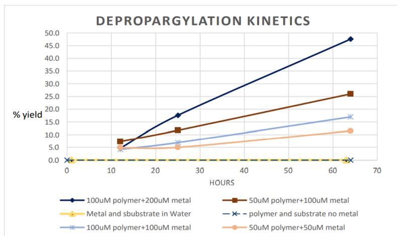
**Figure 5:** Reaction kinetics of depropargylation of 4-Nitrophenyl propargyl ether by catalytic micelles with Pd(OAc)<sub>2</sub> containing core.
